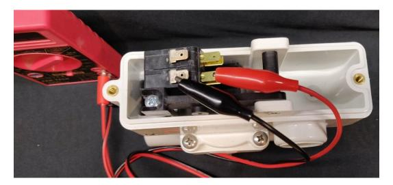
Top two pins of one microswitch out of two microswitch in 220V model.
