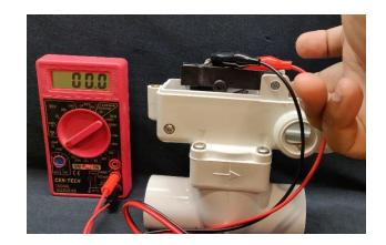
➤ To add more safety to the settings, move the settings screw half turn out (anti clock direction or counterclockwise as shown by the blue arrow on this page.)
